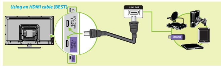
Multi-purpose jacks: You can plug any device that uses HDMI into either HDMI jack. However, certain devices must be connect to the **ARC** or **MHL** jack. See the instructions that came with your ARC, DVI, or MHL device for more information.
